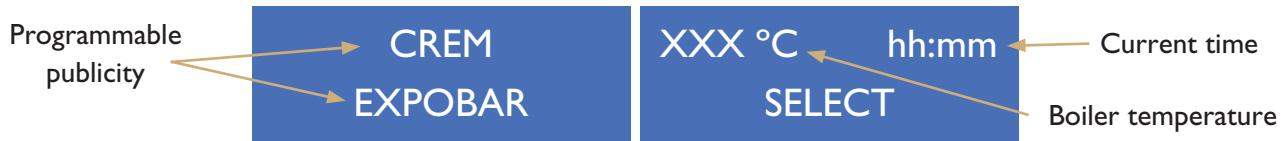
Machines equipped with a display inclPCSe the following additional functions:
